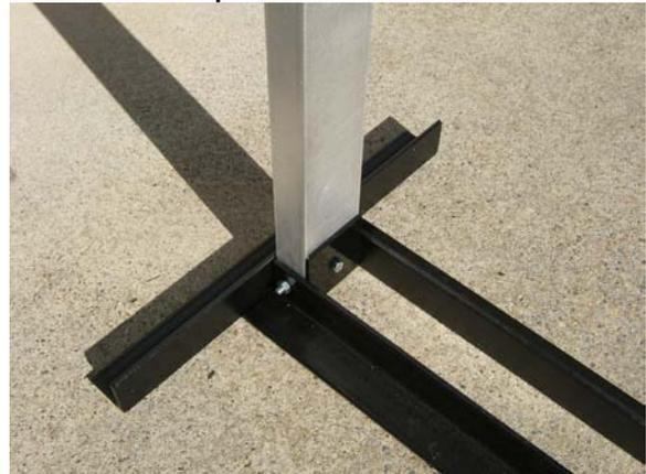
The tree extension is attached to the base stand using the (2) 5/16-18 x 1 inch Hex Head cap screws and nuts. It is easiest to have the nuts on the outside for tightening purposes. The flat steel plate stiffens the front of the tree when the cross bar is tightened. The 2 ½ inch long 5/16-18 is placed through the flat stock, through the tree, and then through the cross bar and fastened with a nut. The cross bar is used to tilt the tree to make it level when on uneven ground.
