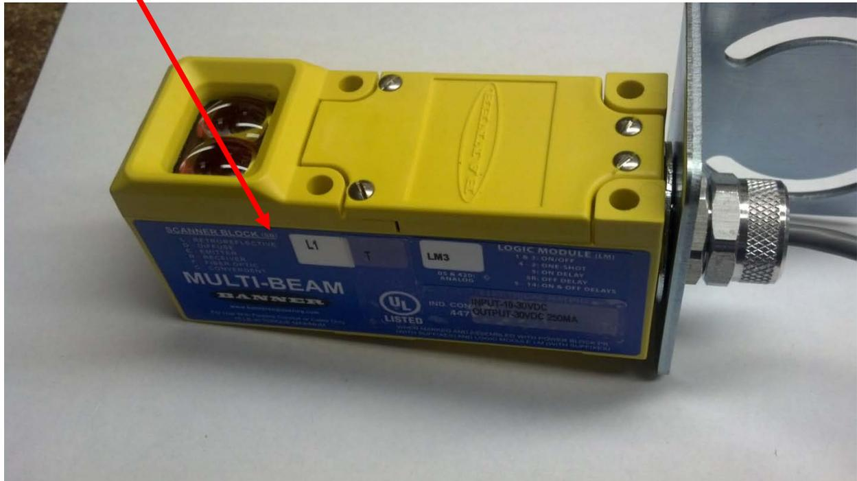
First disconnect the sensor from the track (power). Failure to do so will damage the sensor. Remove cover. The polarity pin should be taped under the cover.
