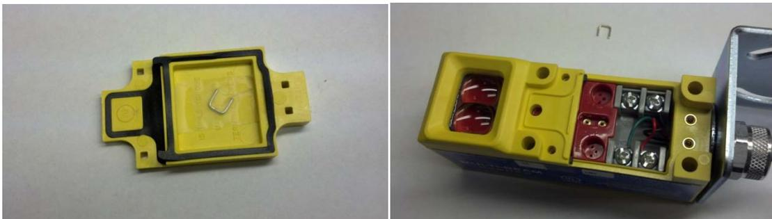
Insert the pin into the two brass holes located in the logic module. The sensor is now set to “HI” polarity.
